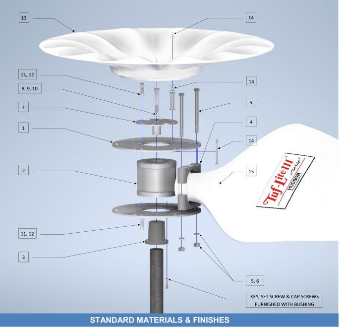
Blades: Fiberglass reinforced vinyl-ester or epoxy Hub Spool: Ductile Iron, Zinc Rich Coating Plates: Steel, Galvanized Bushing: Malleable Iron Seal Disc: Fiberglass Reinforced Polyester
